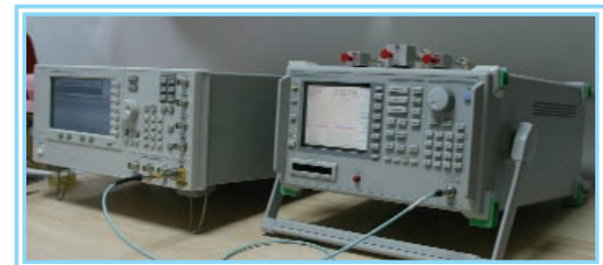
The frequency generator (Agilent) up to 110 GHz purchased in the frame of the European FP7 project MIMOMEMS together with the spectrum analyser (Anritsu)
