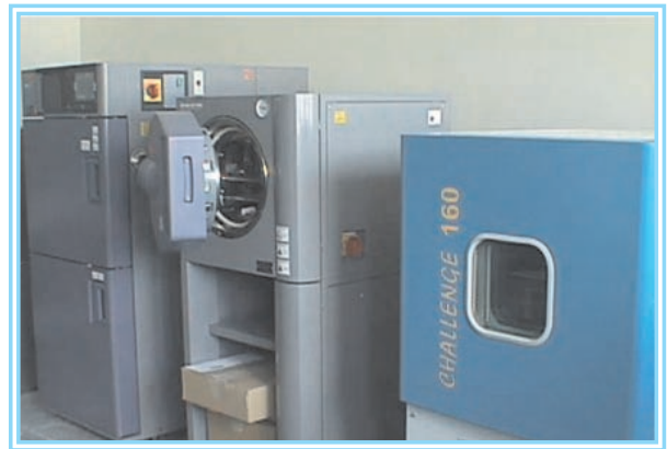
Chambers for: -Thermal cycling – TSE-11-A (Espec): High temp. (-65...0°C) and Low temp.(+60...200°C); -Highly accelerated stress test (HAST) - EHS 211M (Espec): Temperature range: +105 ... +142°C, Humidity range: 75%...100% RH, Pressure range: 0.02...0.196 Mpa; -Damp heat - CH 160 (Angelantoni)
