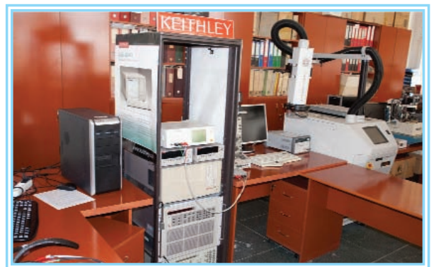
Electrical characterization: 4200SCS system Keithley, UK.
