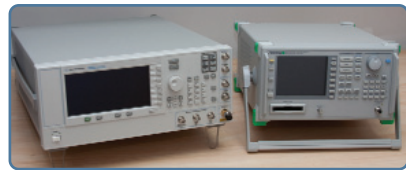
Upgraded to 110GHz set-up for "on wafer" S parameters measurements (top), Generator up to 110 GHz and the Spectrum Analyzer up to 110 GHz (bottom).
