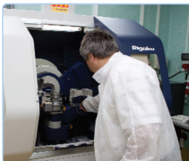
Mihai Danila (mihai.danila@imt.ro) introducing in the sample in the XRD for investigation the Pt nanocrystallite orientation and size
