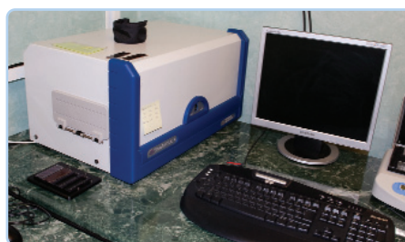
Monica Simion ( monica.simion@imt.ro ) working on the Micro Plotter to prepare a protein C reactive microarray slide
