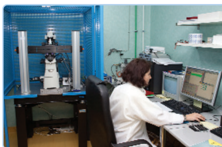
Mihaela Miu ( mihaela.miu@imt.ro ) investigating the electrocatalytic activity of the gold nanoparticle electrode array with SECM
