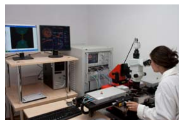
"on wafer" characterization equipment up to 110 GHz.
