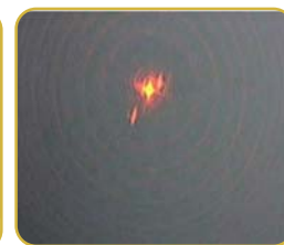
Reflected light in the focal plane: Fresnel lens with 4 levels
