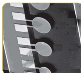
SEM image of micromirrors with circular and rectangular geometry obtained on silicon substrates
