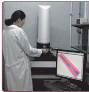
The installed white light interferometer and a resulting 3D image of a membrane supported Schottky diode
