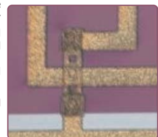
Detail of the air bridge of the membrane supported spiral inductor
