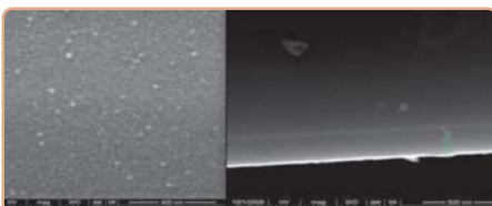
SEM surface and cross section images of the ZnO (Zn 0,05 M 1) film, formed by 4 successive sol-gel deposited films, annealed in air at 500°C, 1h.
