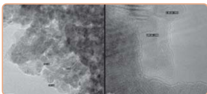
Bright Field HR-TEM images of ZnO thin film deposited by DC magnetron sputtering from Zn target and further oxidized in air at a temperature of 450°C for 3h. The nano-crystallites size is less than 20nm, are (100) and (002) oriented, and their structure is wurtzite.
