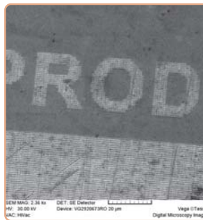
SEM micrographs of authentication stamps used in food industry.
