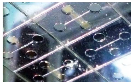
Microfluidics device encapsulated with borosilicate glass
