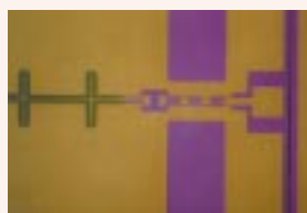
77 GHz hybrid receiver based on silicon micromachining (design: IMT-Bucharest; manufacturing: ITC-Trento)
