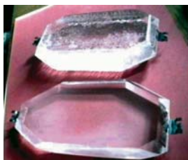
a-SiO 2 single crystals obtained by hydrothermal synthesis (details in MNT-Bulletin V3, no.3)
