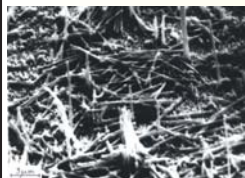
SEM on Ni_{80}Fe_{20} nanowire array after dissolution of the membrane (details in MNT-Bulletin V3, no.4)
