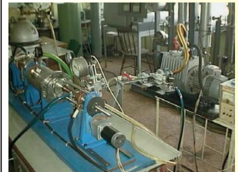
Production of the fullerene soot with C60-C70 mixture; the extraction of C60-C70 mixture, their separation and analysis by FT-IR spectroscopy (details in MNT-Bulletin V2, no.2-3)
