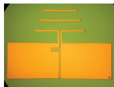
35 GHz micromachined Yagi antenna structure
