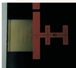
Bottom view of "quasi three edges" Yagi Uda membrane supported antenna structure
