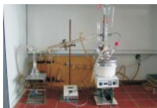
Laboratory glass equipment for work in inert atmosphere (manifold for inert gas, adapted standard glassware)
