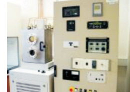
Sputtering system 5Pascal: For magnetron sputtering of conductive materials (Au, Pt, Cr, Cu, Ti etc.) and glow discharge plasma cleaning of surface.
