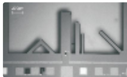
Silicon monocrystalline cantilevers of different shape, 15µm thick.
