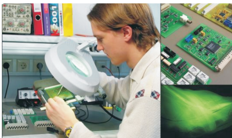
Left: Development of electronic circuits for electroporation devices. Top right: Printed circuit boards designed in our laboratory. Bottom right: Green fluorescent protein (GFP) fluorescence after successful insertion of the GFP reporter gene into muscle cells by means of electroporation.
