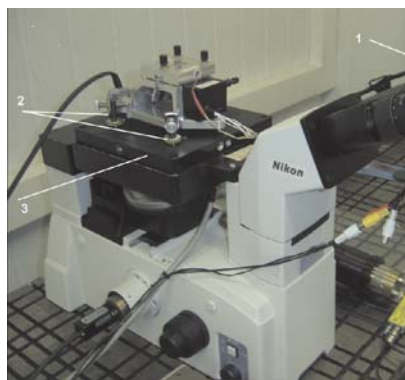
Biological AFM combined with inverse optical microscope and possibilities for single cell manipulation.
