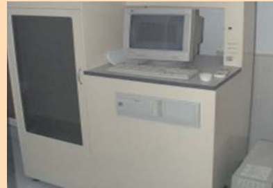
Laboratory of Rapid Prototyping and Reverse Engineering Laser stereolithograph LS 250 [NICTL Shatura] using LGK 30 He/Cd laser, filled with Renshape/Cibatool SL 5170 epoxy resin, default layer thickness 0.1 mm.
