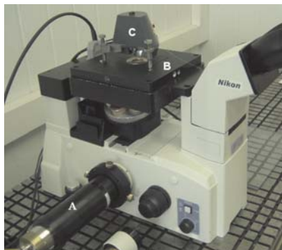
Scanning Near Field Optical microscope with photon counting and fluorescence imaging
