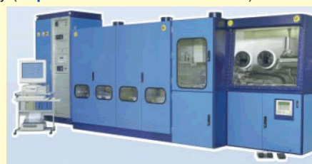
MOCVD (Metal Organic Chemical Vapor Deposition) System
