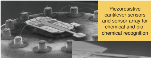
Piezoresistive cantilever sensors with ultra sharp tips
