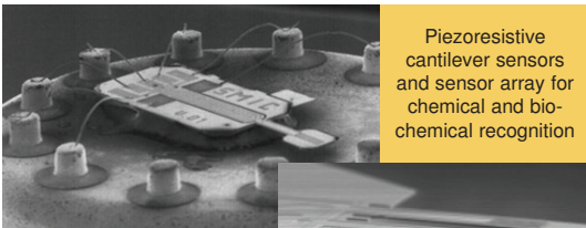
Piezoresistive cantilever sensors with ultra sharp tips
