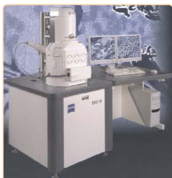
"Scanning Electron Microscope (SEM) with energy dispersive detector for X-rays (EDX) and with an option of Electron Beam Lithography (EBL).
