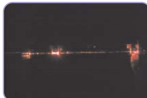
7.5 \mu\text{m} wide straight WG leaky-wave coupled with a Si photodiode, optical images and light propagation
