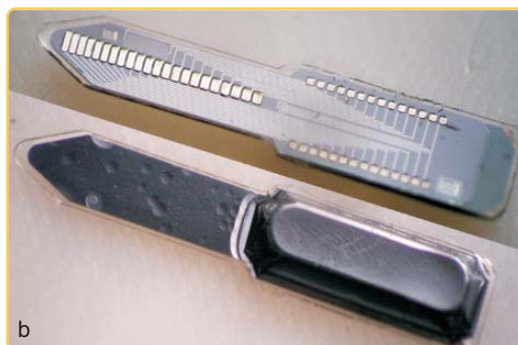
Fig. 2 Examples of electrodes for hearing implants: a) passive cochlear microelectrode containing 22 Pt stimulation sites coated with silicone rubber, b) silicon modiolus electrode integrated with a piezoresistive deflection sensor and protected with parylene-silicone coating
