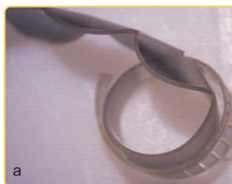
Fig. 2 Examples of electrodes for hearing implants: a) passive cochlear microelectrode containing 22 Pt stimulation sites coated with silicone rubber, b) silicon modiolus electrode integrated with a piezoresistive deflection sensor and protected with parylene-silicone coating
