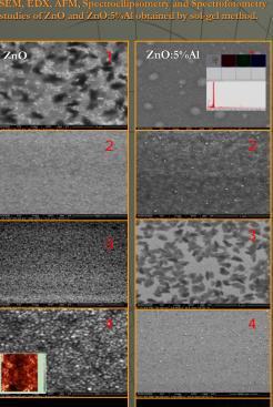
Evolution of ZnO and ZnO:5%Al thin films morphology. The films have been obtained by deposition of 4 succesive layers using sol-gel method. Each layer was treated after deposition at 500°C in ambient atmosphere for 1 hour.
