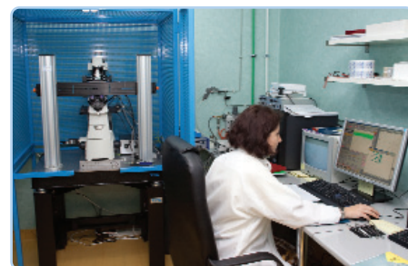
Mihaela Miu (mihaela.miu@imt.ro) investigating the electrocatalytic activity of the gold nanoparticle electrode array with SECM
