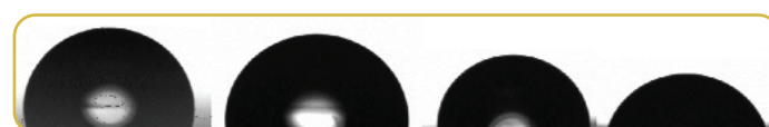
PDMS hydrophilization by plasma treating and contact angle measurements: a) PDMS sample- untreated: contact angle contact 112° , b) PDMS treated in SF6 (P=10Pa, Prf=50W, t=10min, SF6=100scm)- contact angle 105° c) PDMS treated in SF6 (Prf 200W) +O 2 - contact angle 97° d) treatment in SF6 (Prf 250W) +O 2 - contact angle 85°.
