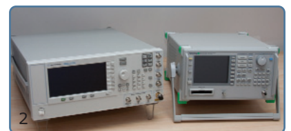
Upgraded to 110GHz set-up for "on wafer" S parameters measurements (left), Generator up to 110 GHz and the Spectrum Analyzer up to 110 GHz (top).
