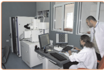
EBL equipment (e-line Ultra High Resolution Electron Beam Lithography and Nanoengineering Workstation)
