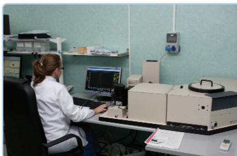
Teodora Ignat (teodora.ignat@imt.ro) investigating a Cy3 labelled DNA sample by fluorescence spectrometry
