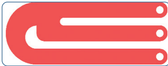
Curved microfluidic filter, for cell separation depending on size and weight.
