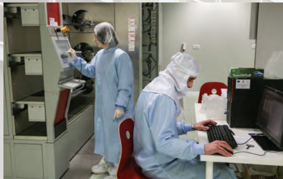
Horizontal oven Centrotherm E1200. R&D equipment for the fabrication of substrate used for electronic devices based on graphene
