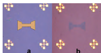
Patterning of graphene channel: (a) in electron resist, (b) after RIE etching
