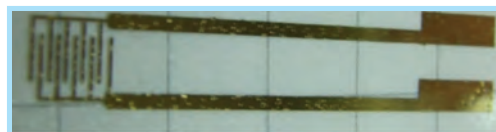
The InkJet-printed Au impedimetric sensor, on PET substrate
