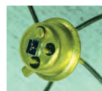
FET transistor with nanostructured graphene channel, after wire and die bonding
