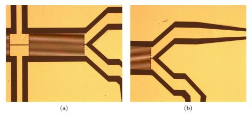
Fig. 2. Microscope photos of the fabricated coupler. Details for the interdigital capacitors and the CPW stubs area (a) and for the tapered CPWs area (b).
