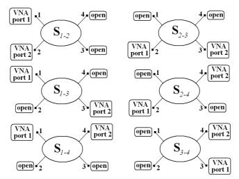
**Fig. 1.** The possible 6 combinations of two-port measurements (using a two-port VNA), for a four-port circuit.
