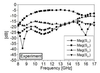
**Fig. 3.** Experimental scattering parameters, for the 4-port test circuit (a coupler).
