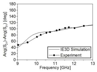
Fig. 5. Simulated and experimental phase difference between the coupled port and the through port of the coupler considered as a test 4-port circuit.
