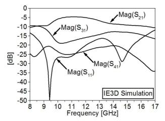
**Fig. 4.** Simulated scattering parameters, for the 4-port test circuit (a coupler).
