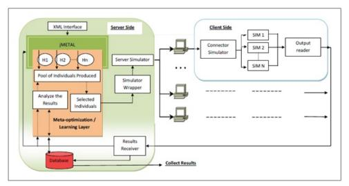
Fig. 1. Structure of FADSE (distributed version).
