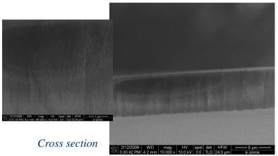
SEM images of nanoporous porous silicon (nanoPS) obtained by electrochemical porosification of Si substrate
