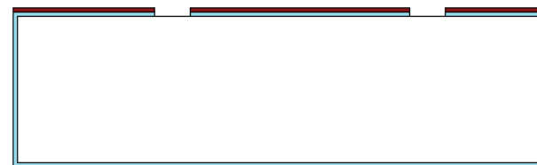
Resist deposition and patterning; SiO2 dry etching
