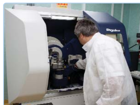
Mihai Danila (Mihai.danila@imt.ro) introducing in the sample in the XRD for investigation the Pt nanocrystallite orientation and size
