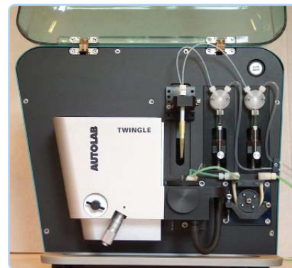
Autolab TWINGLE - Dual Channel E-SPR
