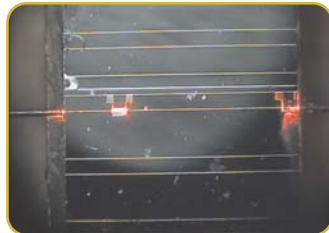
7.5 \mu\text{m} wide straight WG leaky-wave coupled with a Si photodiode, optical images and light propagation
