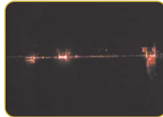
7.5 \mu\text{m} wide straight WG leaky-wave coupled with a Si photodiode, optical images and light propagation
