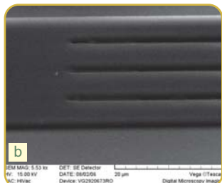
Polymeric multimode-interference (MMI) waveguide couplers: a), b) SEM images; c) light propagation
