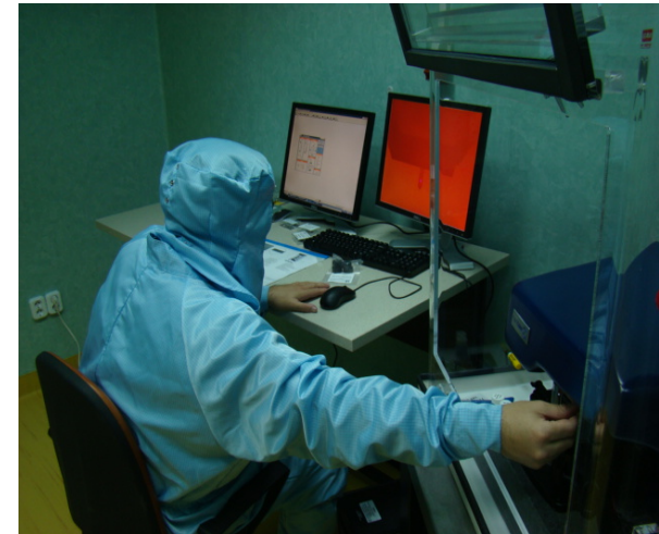
Setting-up the system. Left monitor: used for working with the CAD-like software that controls the system; right monitor (orange): real-time imaging of the cantilever tip; extreme right (blue): the NScriptorTM system The window of the environmental chamber is open
