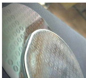
Lentila Fresnel \phi = 20 \mu\text{m} Detaliul minim: 3 \mu\text{m}
