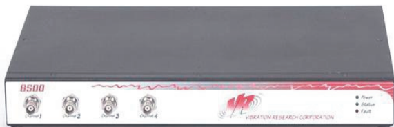
Controller Vibration Research Corporation VR8500
