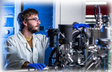
X-ray photoelectron spectroscopy (XPS) PHI 5000 VersaProbe II („XPS scanning microprobe“)
