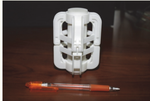
Beta version of the torque sensor (sensor part) made by Selective Laser Sintering of polymer (polyamide PA2200)
