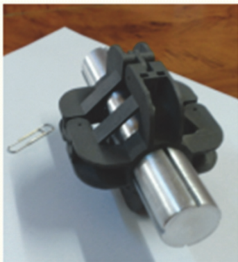
Torque sensor mounted on a metallic shaft (not final shaft)
