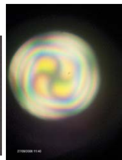
Photo of the Malta cross in a quartz sample, in monochromatic and white light respectively. The arms of the cross are curved because of the optical rotatory power of the quartz. Crystal thickness of 3.9 mm.
