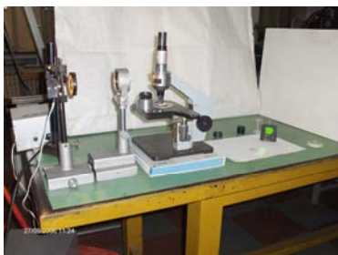
Photo of an experimental model of the reflective conoscope, developed in cooperation by IMT-Bucharest and S.C. ProOptica S.A.
