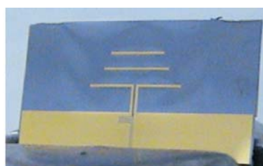
A test F-BAR structure on GaN membrane, IMT, TUD, FORTH (Proc. of MEMSWAVE 2005 Workshop, Lausanne, pp. 63-66)
