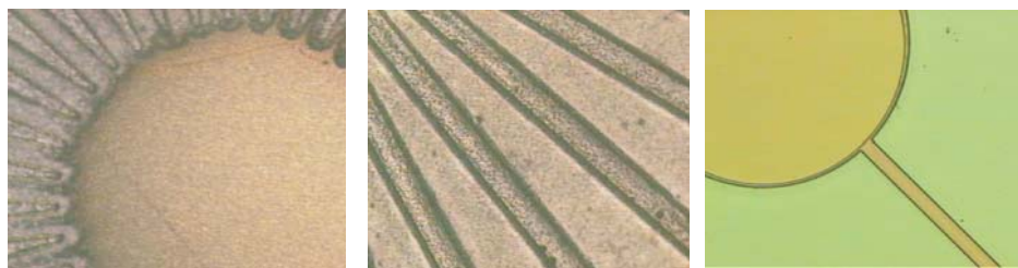
Micro-heat sink based on silicon surface microprocessed Au microchannels.
