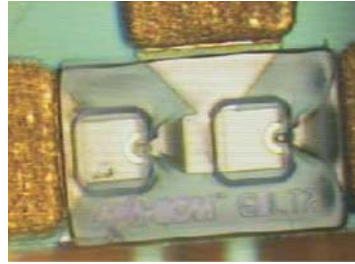
Image of receiver structure with membrane supported Yagi Uda antennae, hybrid integrated with an antiparallel GaAs Schottky diode pair - IMT, LAAS (Proc. IEEE Int. Workshop on Antenna Technology - IWAT 2005, pp. 113-116)
