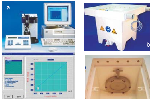
VOLTALAB10 and Trace Master 5 (a); AMMT: Wet etching system for 4' silicon wafers (b);
