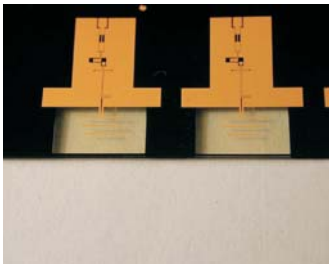
Image of receiver structure with membrane supported Yagi Uda antennae, hybrid integrated with an antiparallel GaAs Schottky diode pair - IMT, LAAS (Proc. IEEE Int. Workshop on Antenna Technology - IWAT 2005, pp. 113-116)
