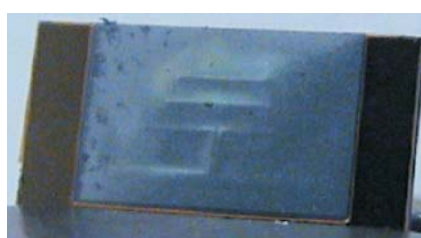
Photos of the 45 GHz membrane supported Yagi Uda antenna, top view (left) and bottom view (right) - IMT, FORTH, (Journal of Micromech. Microeng., vol.15, No. 7, pp. S53-S59, 2005)
