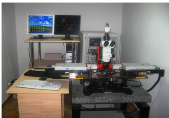
VNA ANRITSU 37397D (up to 110 GHz) with Karl Süss on wafer characterization system
