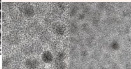
HRTEM: \text{Nd}_{50}\text{Fe}_{40}\text{Al}_{10} melt-spun ribbon thickness: 25 mm HRTEM: \text{Nd}_{50}\text{Fe}_{40}\text{Al}_{10} melt-spun ribbon thickness: 120 mm
