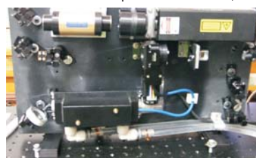
Fig. 2. Frequency doubled (532 nm), microchip laser oscillator-amplifier, manufactured by NILPRP
