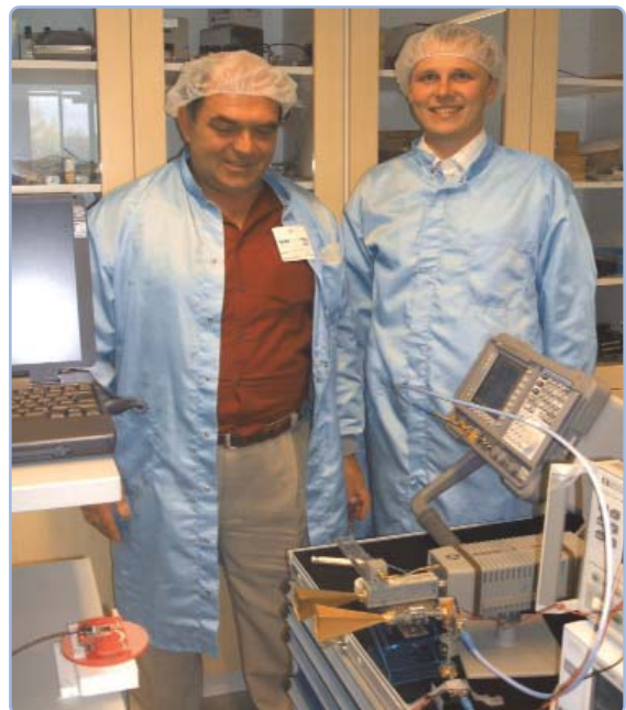
Fig. 2 Dr. Alexandru Müller (IMT-Bucharest) and Dr. Tauno Vähä-Heikkilä (VTT- Helsinki), testing the 60 GHz receiver, used in the first millimetre wave identification (MMID) tag developed in Europe.
