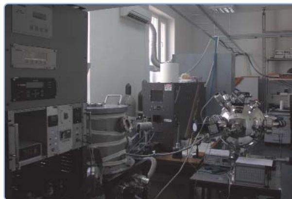
Fig. 1: Pulsed Laser Deposition facility in operation in LSPI Laboratory
