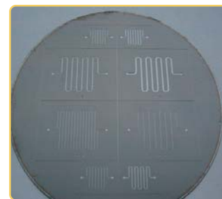
Fig.1. Silicon wafer with microchannel structures
