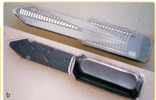
Fig. 2 Examples of electrodes for hearing implants: a) passive cochlear microelectrode containing 22 Pt stimulation sites coated with silicone rubber, b) silicon modiolus electrode integrated with a piezoresistive deflection sensor and protected with parylene-silicone coating
