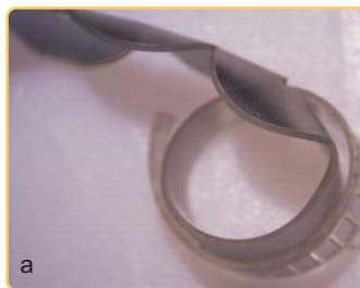
Fig. 2 Examples of electrodes for hearing implants: a) passive cochlear microelectrode containing 22 Pt stimulation sites coated with silicone rubber, b) silicon modiolus electrode integrated with a piezoresistive deflection sensor and protected with parylene-silicone coating
