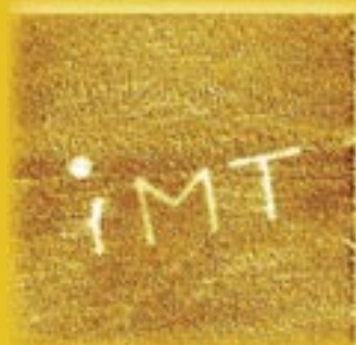
Image size is of 5 microns x 5 microns, the width of the letters is of 115 nm while the dot on "i" radius is of 180 nm. Substrate used is gold and the text is written with MHA (16 - Mercaptohexadecanoic Acid). The image was read at an angle of 10 0 . The text represents the logo of the National Institute of Microtechnology - Bucharest.
