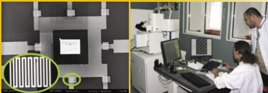
The figure also shows mix-and-match lithography for biomedical applications: optical lithography (left)
