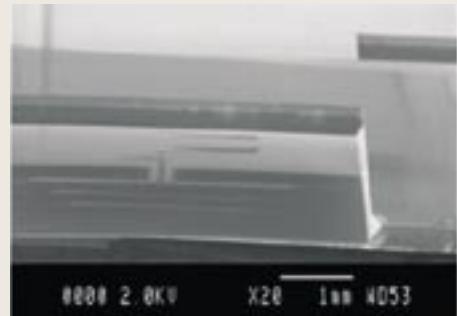
Figure 1: Membrane supported Yagi Uda antenna membrane obtained by silicon micromachining – (common work of IMT and LAAS-CNRS Toulouse).
