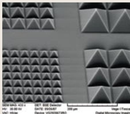
Figure 2 above, figure 3 below: Polymer-based diffractive optical elements obtained by replication PMMA DOE's (above), PDMS microlenses (below)
