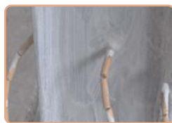
Experiment for measuring the insulating effects of paint; the foaming of the paint exposed to high temperature
