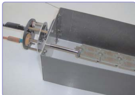
Equipment for testing at tilting & temperature of MEMS accelerometers
