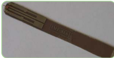
Pen-shape microprobe mounted on an electrical board
