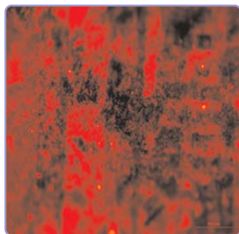
The surface of working micro-electrode. Image at epifluorescence microscope (x10)
