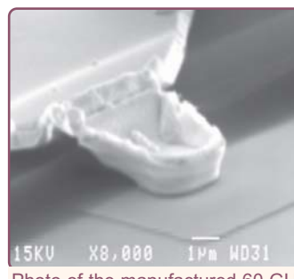
Photo of the manufactured 60 GHz receiver structure for the MMID tag and a SEM detail with of the Schottky diode (IMT, FORTH) - Proc of the SPIE Conf on Smart Materials Nano and Microsystemms 10 -13 December Adelaide 2006
