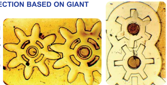
Micromechanical system of gear-wheels microfabricated on polysilicon
