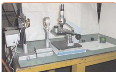
Photo of an experimental model of the reflective conoscope, developed in cooperation by IMT-Bucharest and S.C. ProOptica S.A.
