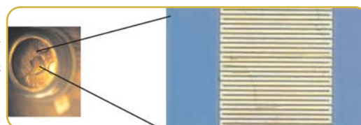
Optical image of a MSM-PD with transparent interdigitated electrodes of ZnO
